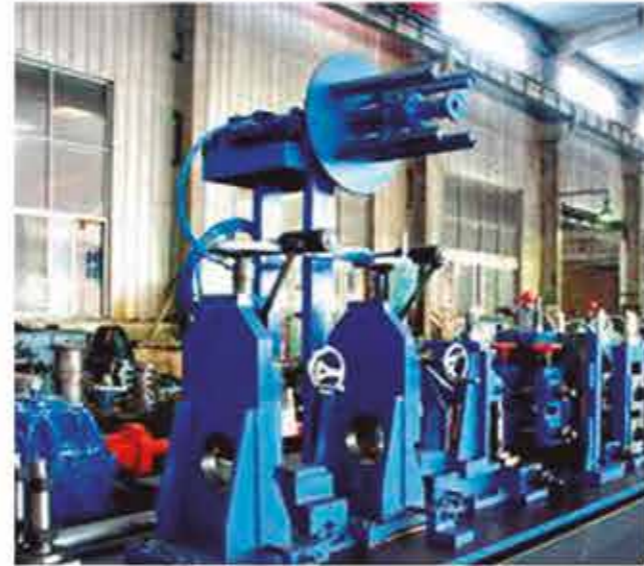
Pelger rolling mill
